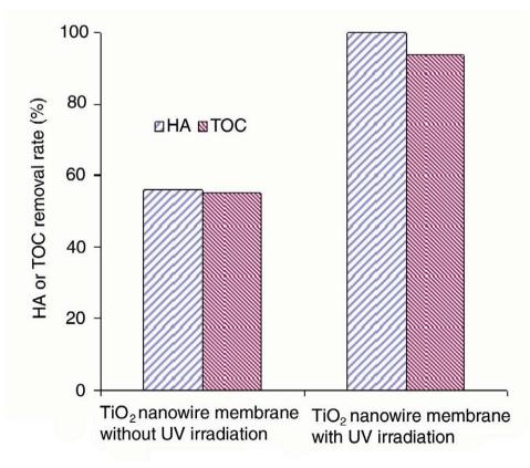
Figure 2: The removal rate of HA and TOC by the TiO2 nanofiber membrane filtration with and without irradiation.
